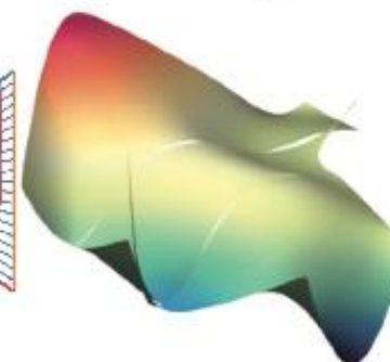
discontinuous stress field ( C^0 multi-patch NURBS) continuous stress field (multi-sided surface)
